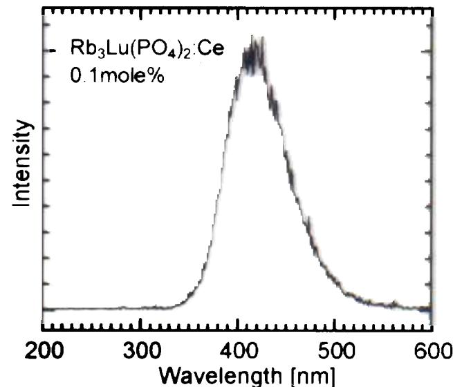
Room temperature X-ray excited luminescence spectrum of  $\text{Rb}_3\text{Lu}(\text{PO}_4)_2$ : 0.1 mole % Ce. Scintillation properties measurements compare very favorably to those of the best commercial scintillators. Light yield at a level of about 250 % of BGO LY. The maximum intensity at about 410 nm, is suitable for use with light detectors such as photomultipliers with alkali halide photocathodes or avalanche photodiodes.
