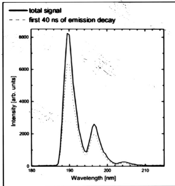
Luminescence Spectrum of Lu(PO<sub>4</sub>):Nd,  $\lambda_{\text{exc}} = 110 \text{ nm}$
