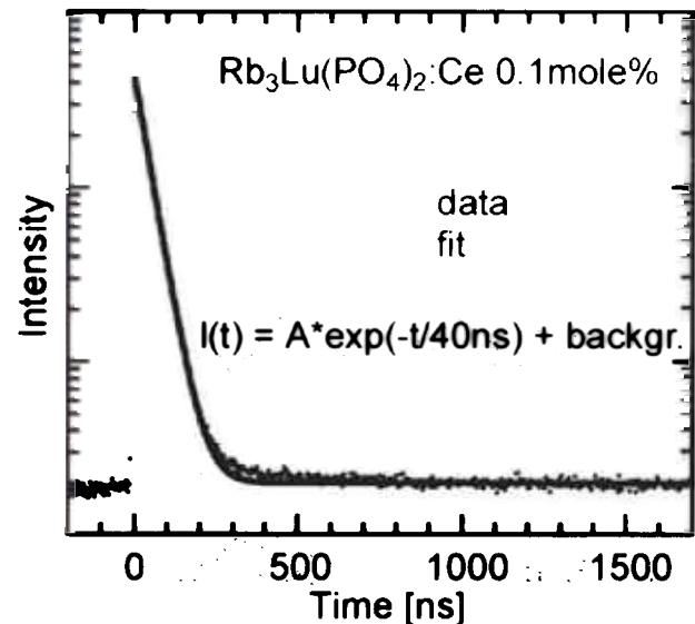
Room temperature scintillation time profile of  $\text{Rb}_3\text{Lu}(\text{PO}_4)_2$ : 0.1 mole % Ce excited by 662 keV gamma photons. The decay of the  $\text{Ce}^{3+}$  emission is practically single exponential and quite fast – decay time constant value is about 40 ns.
