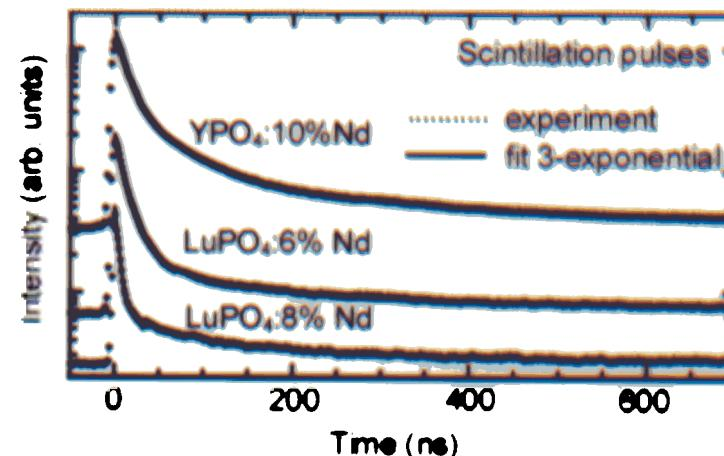
**Selected scintillation pulse shapes of YPO<sub>4</sub>:Nd and LuPO<sub>4</sub>:Nd. Measurements and three exponential fits were done for a 2500 ns time range.**
