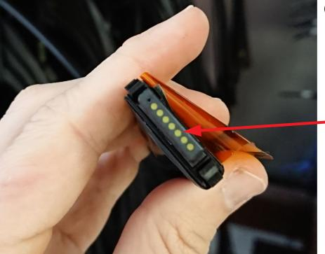
In assembly cleaning was done with ethanol and q-tip
