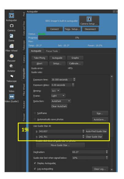
After verifying that the guiding is working, from the position of the guide star in these images, you are ready to observe your target. We recommend doing so with TheSky > Camera > Take Series. Don't forget to set up Autosave. Save your images on the TCS, in an appropriate directory and with recognizable and meaningful filename prefixes.
