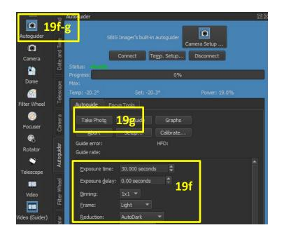
i. If the guide star does appear, and is in an OK position on the autoguider CCD, **double-click on it** to select it for guiding. Verify that its pixel coordinates appear in the **TCS > Autoguider** pane.
