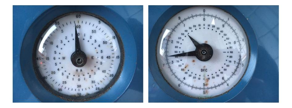
**Step 6a**: dial readings with the telescope at zenith. Left: HA = not quite 1m W. Right: Dec precisely 42 42'.
