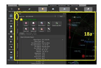
g. Draw a small subframe around your star: **TheSky FITS Viewer > Draw Subframe** (button). This automatically checks the **Subframe** box in various of the **Camera** tabs.
