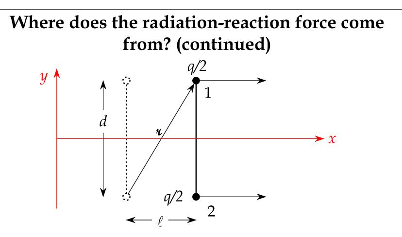
Consider two charges q/2, separated by distance d and moving as shown, but instantaneously at rest ( $v = 0, a \neq 0$ ) at retarded time  $t_r$ . Find the total force: the sum of the forces of each on the other, in the limit  $d \rightarrow 0$ .
