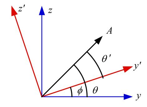
The coordinates of vector A in coordinate system S are related to the coordinates of vector A in coordinate system S':
