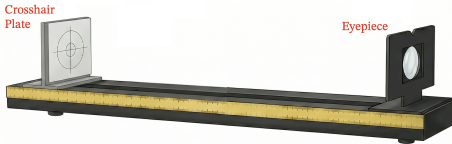
Figure 6: The setup for testing the magnification of a converging lens.
