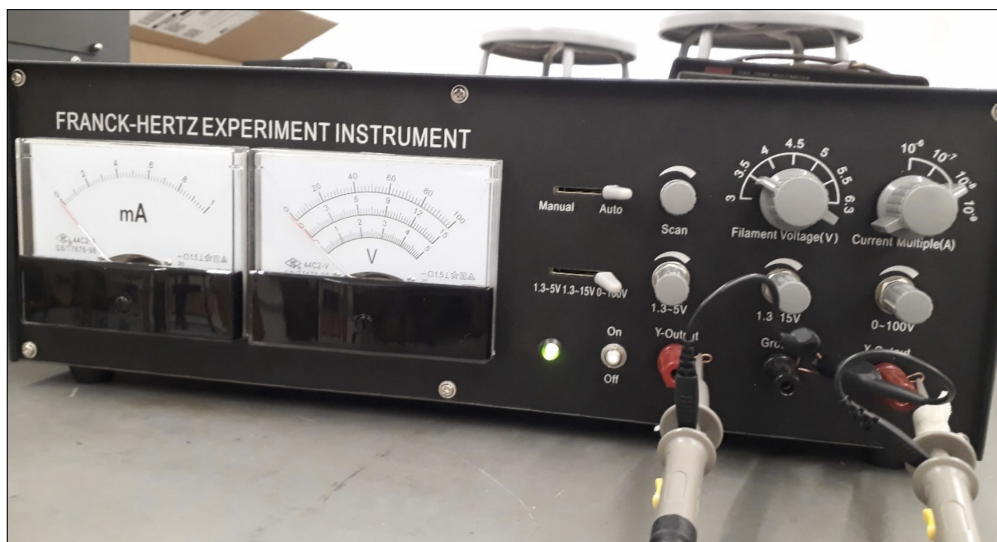
Figure 7: Oscilloscope probe connection to the voltage panel of the Franck-Hertz kit.
