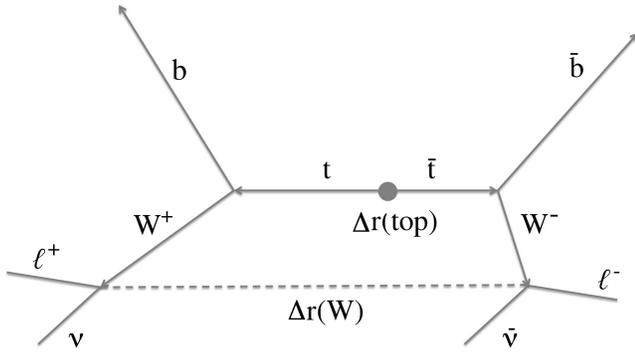
FIG. 1. Schematics of  $t\bar{t}$  production with subsequent decay to  $W$  bosons and  $b$  quarks. Each  $W$  boson then decays to a charged lepton and a neutrino. The distance between the tops' decay is denoted  $\Delta r(\text{top})$ , while the distance between  $W$ 's decay is denoted  $\Delta r(W)$ .
