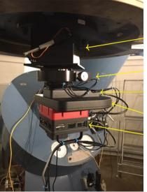
Photometer box, including remote-control camera cover
