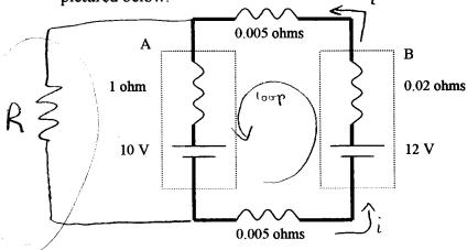
(a) (15 pts) - What is the current in the circuit in the figure? Indicate the direction of the current clearly on the figure.
