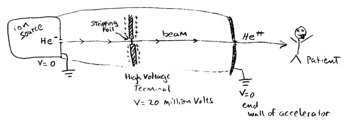
A rather Poor schematic of a tandem van de Graff accelerator
