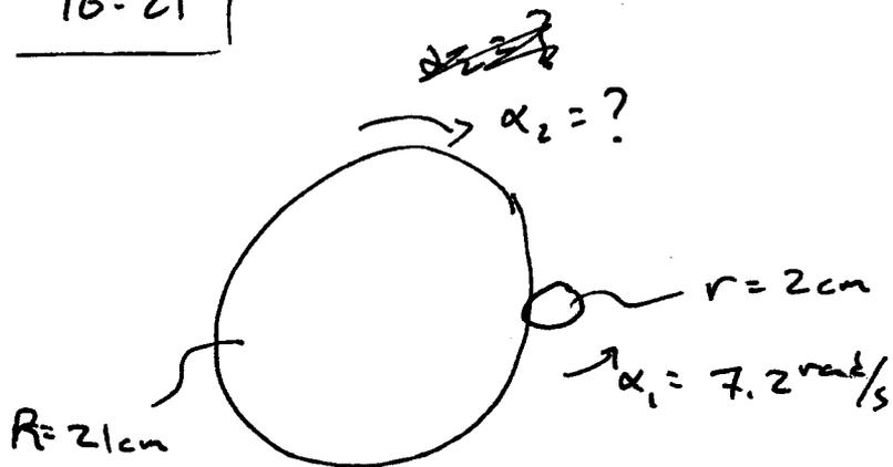
A) SINCE THE EDGES DON'T SLIP WE KNOW THEY MUST HAVE THE SAME TANGENTIAL VELOCITY AT ALL TIMES, AND HENCE, THE SAME TANGENTIAL ACCELERATION.
