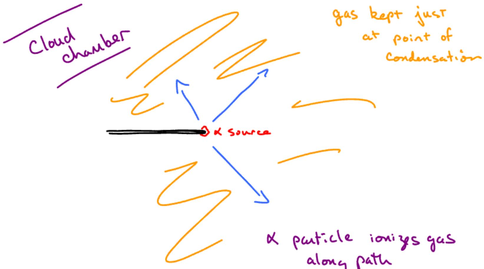
α particle ionizes gas along path
