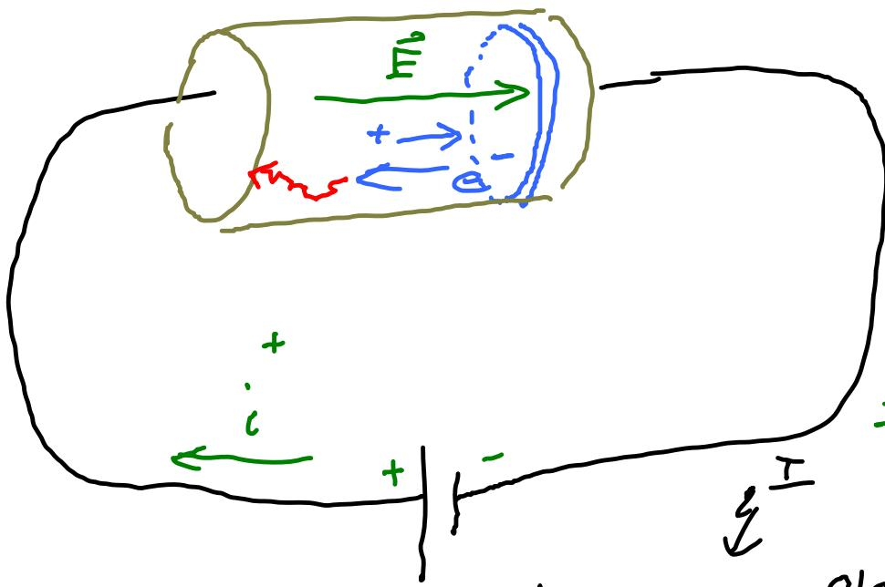
$$\text{charges will flow} = \frac{dq}{dt} = i \equiv \text{current}$$
