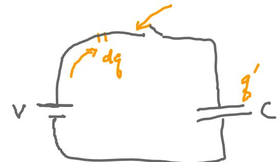
Energy required to charge Capacitor =  $\frac{Q^2}{2C} = \frac{1}{2} CV^2 = \frac{1}{2} QV$
