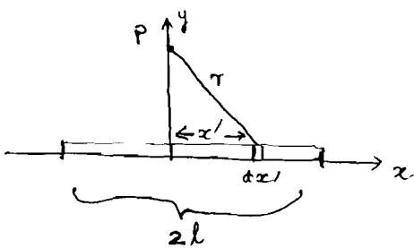
we choose a small length element  $dx'$  at a distance  $x'$  from center of rod and find the potential due to that. Total charge on rod =  $Q$ .
