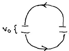
In one circular motion the particle passes through the gaps twice. Hence net increase in energy is  $2qV_0$ .
