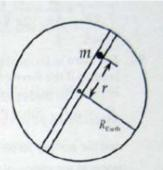
$$m_r = \rho V_r = \frac{M_{\rm Earth}}{V_{\rm Earth}} V_r = \frac{M_{\rm Earth}}{\frac{4}{3}\pi R_{\rm Earth}^3} \frac{4}{3}\pi r^3 = M_{\rm Earth} \frac{r^3}{R_{\rm Earth}^3}$$
