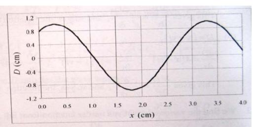
$$D(0,0) = A\sin\phi \rightarrow 0.80 \text{ cm} = (1.00 \text{ cm})\sin\phi \rightarrow \phi = \sin^{-1}(0.80) = 0.93$$
