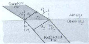
diameter and the interface is equal to the incident and refracted angles. Since the air-glass interface creates the hypotenuse for both triangles we use the definition of the cosine to solve for this length in each triangle and set the lengths equal. The resulting equation is solved for the diameter of the refracted ray.
