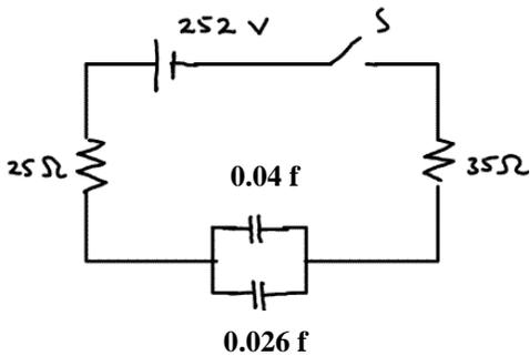
In the circuit to the left, how much energy is stored in the 0.026 farad capacitor 2 seconds after the switch S is closed?
