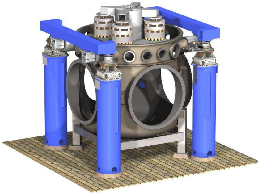
Figure 2.3: BSC Chamber and its seismic isolation
