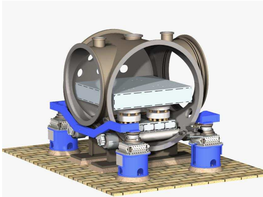
Figure 2.2: HAM Chamber and its seismic isolation
