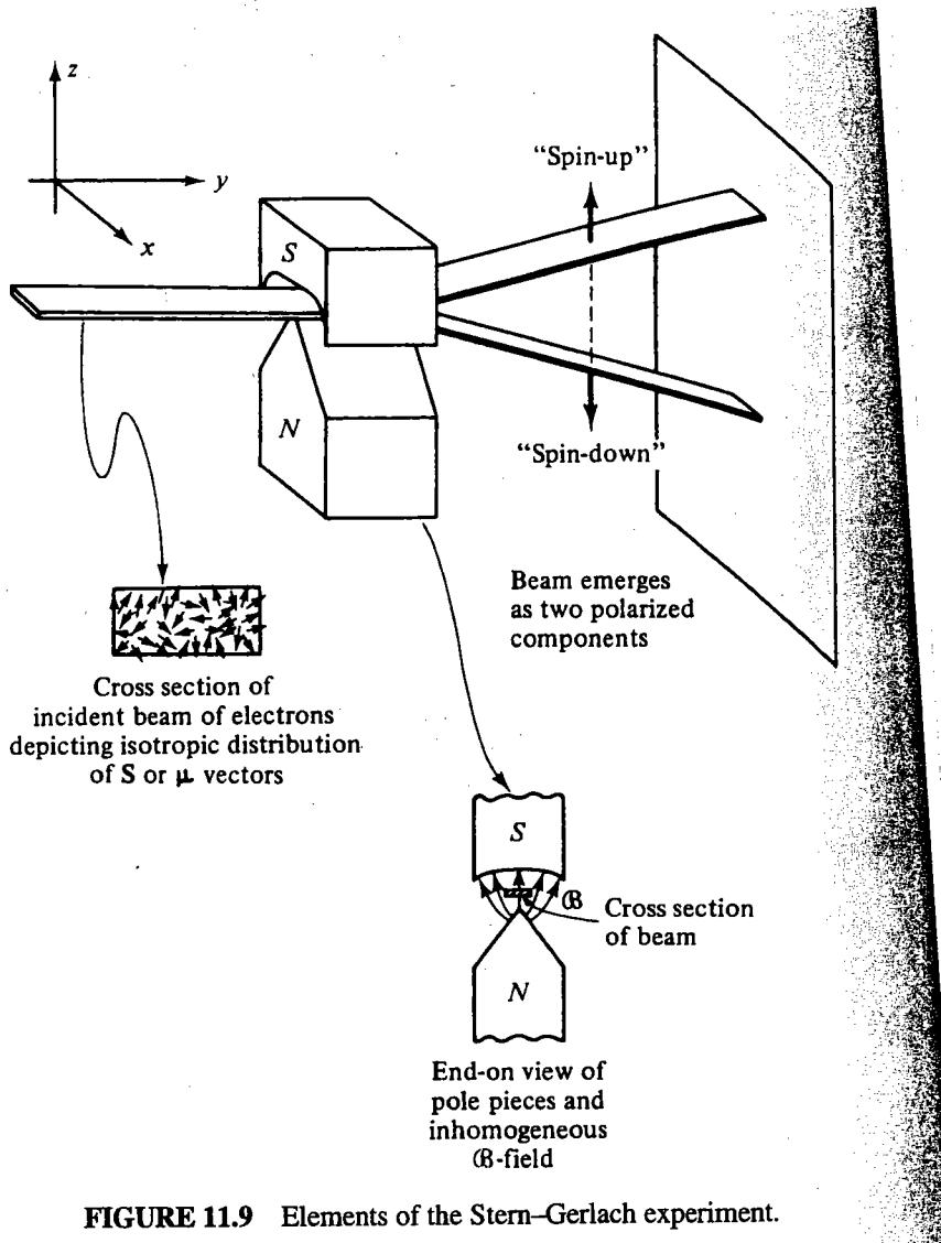
FIGURE 11.9 Elements of the Stern-Gerlach experiment.
