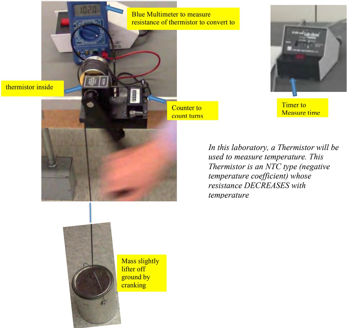
*In this laboratory, a Thermistor will be used to measure temperature. This Thermistor is an NTC type (negative temperature coefficient) whose resistance DECREASES with temperature*
