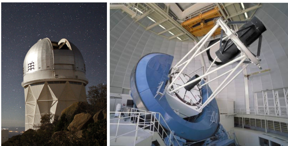
FIGURE 2.1: The Mayall 4-m telescope dome (left) and telescope (right), where the DESI experiment will be conducted. Credit: NOAO.
