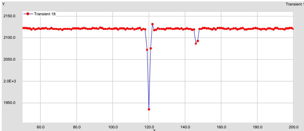
The blue line represents the analog signal, and the red dots represent the digital samples.
