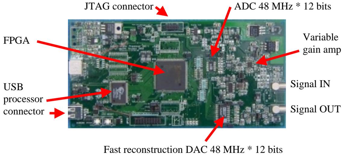
Figure 2. Block diagram of DDC-1.
