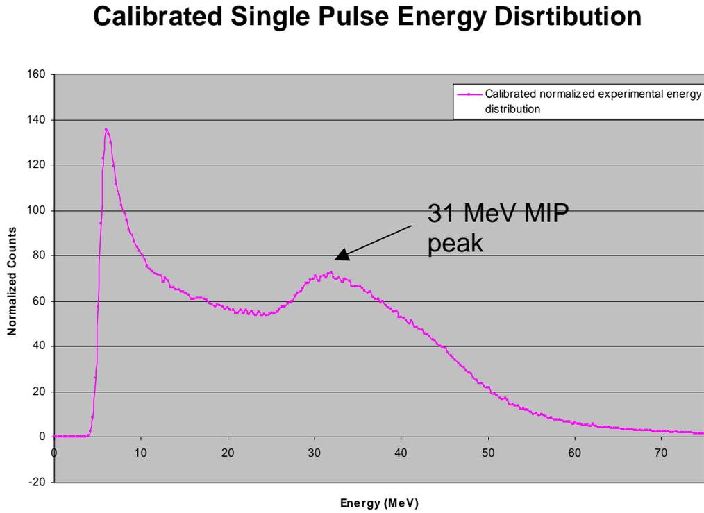
Figure 10. Stopping muon stopping and decay energy distributions
