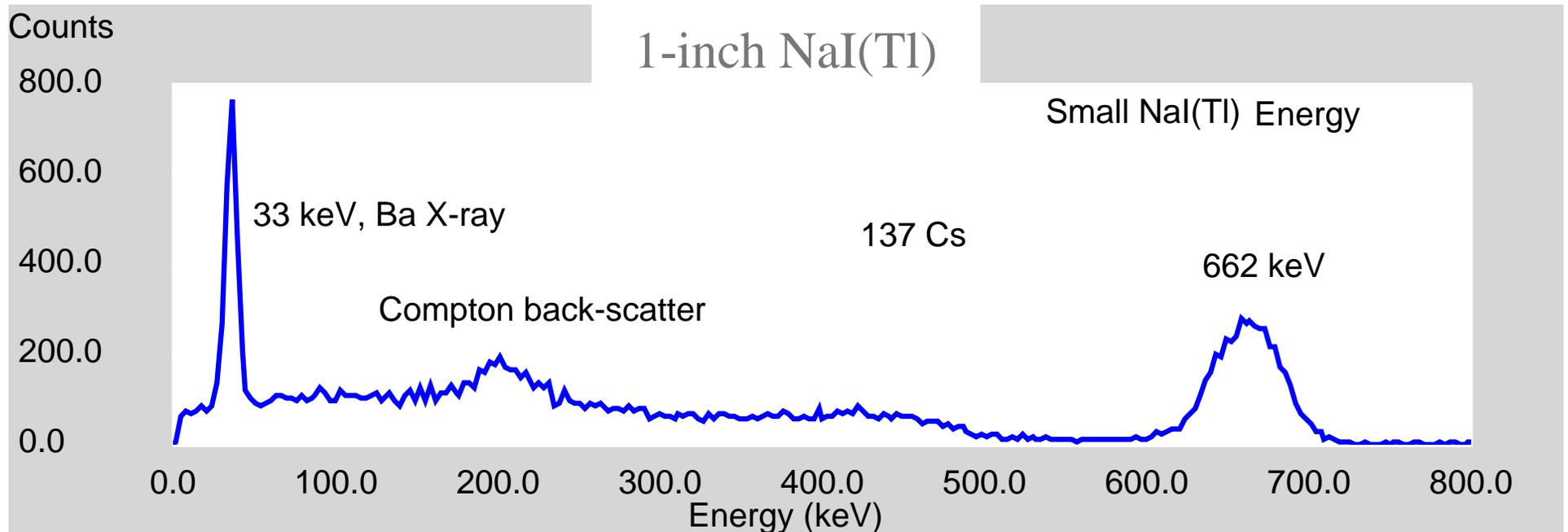
Pulse-height histogram measured with UTM
