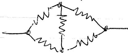
In a resistor, current always flows from the terminal at higher potential (+) to the terminal at lower potential (-).
