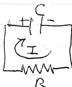
since we take voltage drop across C going clockwise around loop, we should take the direction of I also clockwise to be consistent
