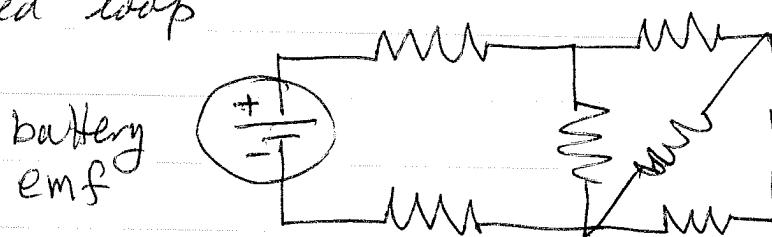
To determine the behavior of the circuit, i.e. how much current flows through each element and what is the voltage drop across each element we have Kirchoff's Laws
