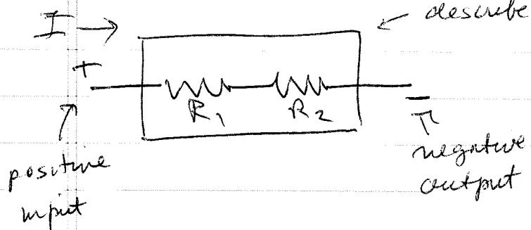
← describe two resistors in series as one effective resistor
