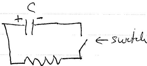
at  $t=0$  capacitor is charged up with  $Q$ . Then switch is suddenly closed. Current will now flow around the loop to discharge the capacitor
