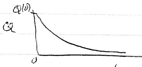
charge on capacitor decays exponentially in time with a time constant  $\boxed{\tau = RC}$
