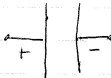
typified by parallel plate capacitor
