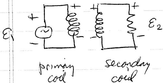
inducting coils configured so that same magnetic flux penetrates each loop of both coils
