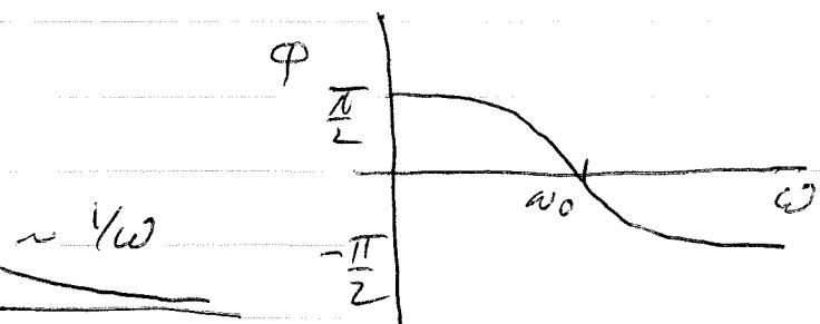
As a measure of the width of the resonance, consider the range of frequencies over which  $I_0$  drops to  $\frac{1}{\sqrt{2}}$  its resonant value
