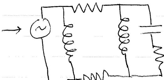
One uses Kirchoff's laws, together with  $I-V$  relationships of each circuit element, to solve for  $I_\varepsilon$  and  $V_\varepsilon$  on each link.
