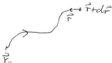
$$= - \int_{\vec{r}_0}^{\vec{r}+d\vec{r}} d\vec{l} \cdot \vec{E} + \int_{\vec{r}_0}^{\vec{r}} d\vec{l} \cdot \vec{E} = \int_{\vec{r}}^{\vec{r}+d\vec{r}} d\vec{l} \cdot \vec{E}$$
