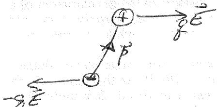
torque tries to align dipole parallel
