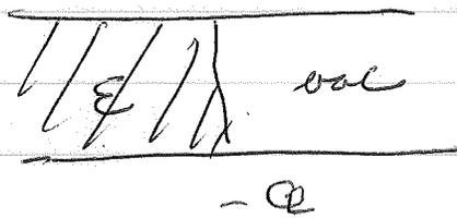
capacitor half filled with dielectric as shown
