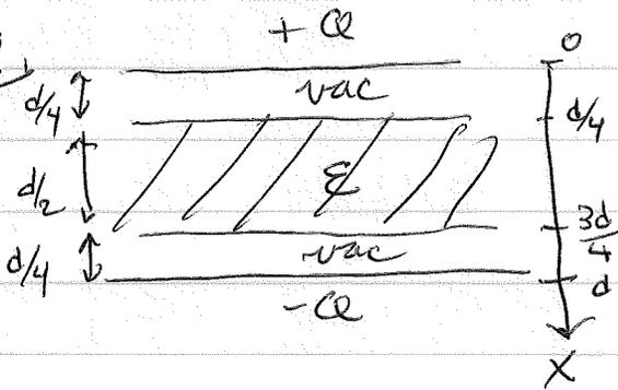
dielectric fills half of space between capacitor plates as shown
