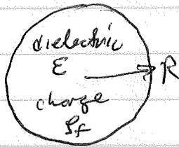
sphere of dielectric with uniform charge density  $\rho_f$  throughout the sphere
