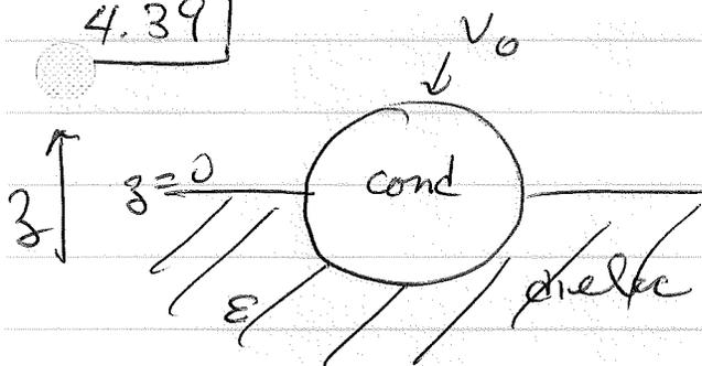
conducting sphere at fixed potential  $V_0$
