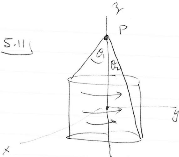
Find  $\vec{B}$  at point  $P$  on  $z$  axis from a solenoid of finite length  $L$ .
