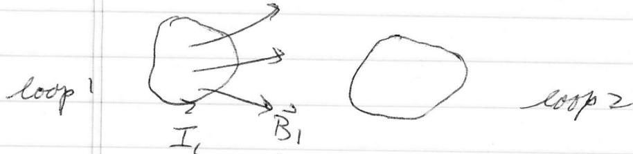
↑ magnetic field due to current in loop 1
