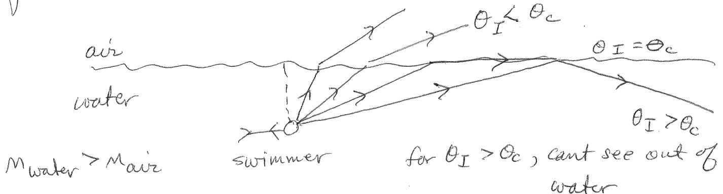
when  $\theta_I = \theta_c$ , transmitted wave travels parallel to interface
