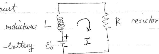
total emf in ~~circuit~~ circuit is:  $E_0 - L \frac{dI}{dt} = IR$  ← Ohms law for the resistor
