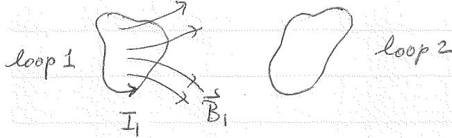
$$\vec{A}(\vec{r}_2) = \frac{\mu_0}{4\pi} \int d^3 r_1 \frac{\vec{I}(r_1)}{|\vec{r}_2 - \vec{r}_1|}$$
