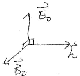
Since Lorentz force is  $\vec{F} = q(\vec{E} + \vec{v} \times \vec{B})$ , the force on a charged particle due to an electromagnetic wave is predominantly from the electric field  $\vec{E}$ . The force due to the magnetic field  $\sim v B_0 = \left(\frac{v}{c}\right) E_0$ , is reduced by a factor  $\left(\frac{v}{c}\right) \ll 1$ , unless charge is moving relativistically fast.
