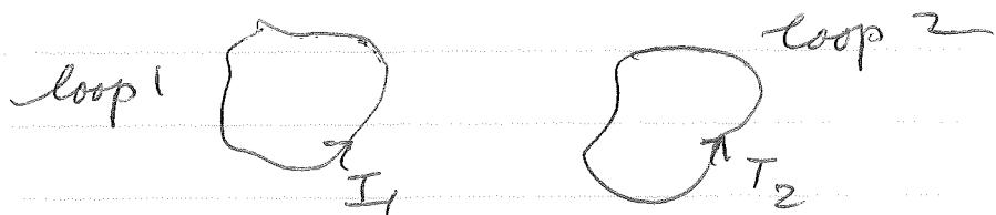
What is the work done to create this configuration of current carrying loops? This will be the energy stored in the configuration. We would like this energy to be independent of the process used to construct the configuration. Loops initially at infinity with  $I_1 = I_2 = 0$ .
