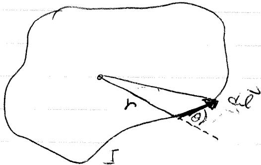
$$\text{area of triangle is } \frac{1}{2} r dl \sin \theta \\ = \frac{1}{2} |\vec{r} \times d\vec{l}|$$
