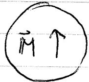
$$\text{bound current} \quad \vec{j}_b = c \vec{\nabla} \times \vec{M} = 0 \text{ as } \vec{M} \text{ constant}$$
