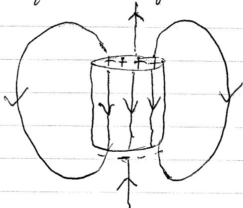
field lines of  $\vec{H}$  = field lines of  $\vec{B}$
