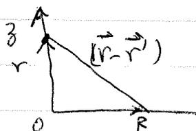
$$\vec{B}(z) = \int_0^{2\pi} d\phi \frac{R}{c} I \hat{\phi} \times \frac{[-R \hat{r} + z \hat{z}]}{(z^2 + R^2)^{3/2}}$$
