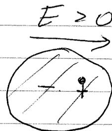
electron cloud and ionic core displaced  $\vec{d} \propto \vec{E}$
