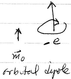
← applying  $\vec{B}$  to orbiting electron slows down its orbital velocity. Net result is again that  $\Delta \vec{m} \propto -\vec{B}$
