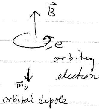
← applying  $\vec{B}$  to orbiting electron speeds up its orbital velocity. Increased angular momentum of negatively charged electron gives change in dipole moment  $\Delta \vec{m} \propto -\vec{B}$
