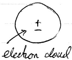
If displace center of electron cloud by a distance  $\vec{r}$ , there is a restoring force  $\vec{F}_{\text{rest}} = -\frac{e^2 \vec{r}}{4\pi R^3} \equiv -m\omega_0^2 \vec{r}$
