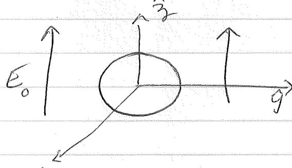
$$\begin{aligned} & \text{boundary conditions} \\ & \left[ \begin{array}{l} \phi(R, \theta) = 0 \\ \phi(r \rightarrow \infty, \theta) = -E_0 r \cos \theta \end{array} \right] \end{aligned}$$
