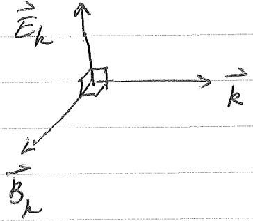
$$\vec{E}_k \perp \vec{k} \quad \vec{B}_k \perp \vec{k} \quad \left. \begin{array}{l} \text{"transverse"} \\ \text{polarization} \end{array} \right\}$$
