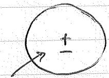
If displace center of electron cloud by a distance  $\vec{r}$ , there is a restoring force  $\vec{F}_{\text{rest}} = -\frac{e^2 \vec{r}}{4\pi R^3} = -m\omega_0^2 \vec{r}$
