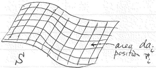
tile surface with infinitesimally small tiles of area  $da_i$  at positions  $\vec{r}_i$  on  $S$
