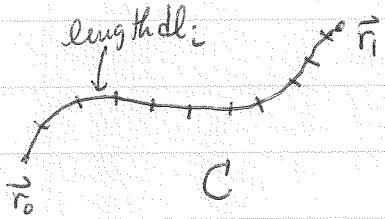
make curve C out of infinitesimally small straight line segments of length  $dl_i$  located at positions  $\vec{r}_i$  on C
