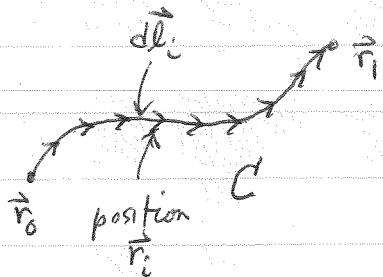
make curve out of infinitesimal displacements  $d\vec{l}_i$ ; direction of  $d\vec{l}_i$  is tangent to C.
