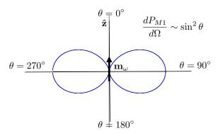
The power distribution is as shown on the left. The distribution is rotationally symmetric about the  $\hat{\mathbf{z}}$  axis. Most of the power is directed outwards into the xy plan  $\perp \mathbf{m}_{\omega}$ .
