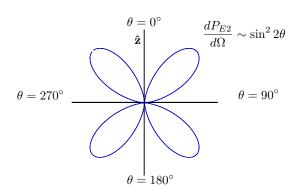
The power distribution is as shown on the left. The distribution is rotationally symmetric about the **2** axis. Most of the powser is directed at  $\pm 45^{\circ}$  to the  $\hat{\mathbf{z}}$  axis.
