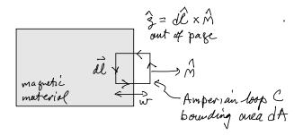
Consider a small Amperian loop C piercing the surface of the material, as shown in the sketch above. The loop C bounds a surface S of area dA whose normal is in the direction  $\hat{\mathbf{z}} = d\hat{\ell} \times \hat{\mathbf{n}}$ , where  $\hat{\mathbf{n}}$  is the outward pointing normal to the surface and  $d\hat{\ell}$  lies in the plane of the surface, as shown in the sketch. Integrate over the surface S, taking the width  $w \to 0$ . One then has,
